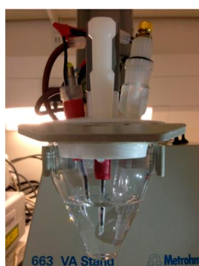
Voltammetric cell with the gold wire, reference and auxiliary electrodes
